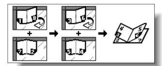
When using the reverse automatic document feeder Spread out the booklet from the middle, and then load it into the reverse automatic document feeder with the front cover at the top.
